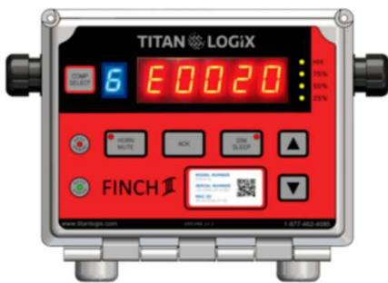
The Error alarm indicates a system error. This alarm can be assigned to the relays and is combined with the SPILL alarm. This alarm will activate the relays when an error occurs on the transmitter or the display. When the cause of the error is resolved, the alarm resets. Since this alarm is self-resetting, no acknowledgment is required for this alarm.
