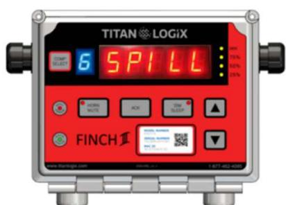
This alarm may be adjusted using Titan Install App. The maximum volume for the Spill alarm is a safety feature that is set at factory and cannot be altered. This alarm may be assigned to relays. If the Spill Alarm level is reached, the FINCH III Display flashes “Spill” and the last known volume; any relays assigned to the Spill alarm will respond.
