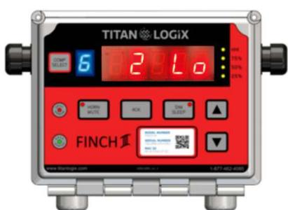
The FINCH Display can show the low level within the bottom dead band by flashing “2 Lo” and the estimated volume. The FINCH Display shows estimated tank volume to the top of the shorting block (2 ½” minimum from the bottom of the tank).
