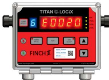
The FINCH III will display error codes when an issue is detected with the system. The Error alarm indicates a system error. This alarm can be assigned to the relays and is combined with the SPILL alarm. This alarm will activate the relays when an error occurs on the transmitter or the display. When the cause of the error is resolved, the alarm resets. Since this alarm is self-resetting, no acknowledgment is required for this alarm.
