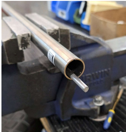
Figure 1 Deburr cut end of tube
