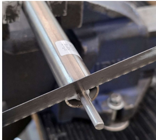
Figure 3 Cut center signal rod flush with end of tube
