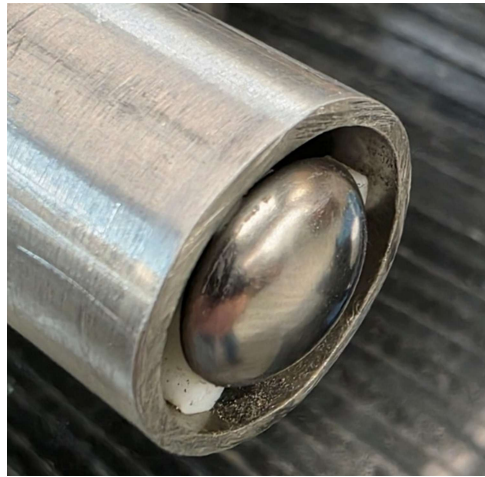
Figure 5 End cap installed on center rod
