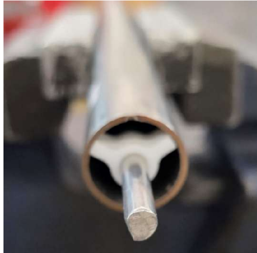
Figure 2 Install Teflon spacer flush with end of tube
