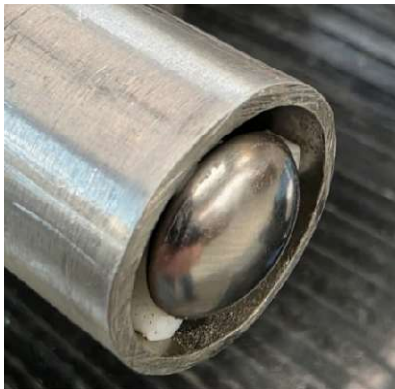
Figure 5 End cap installed on center rod
