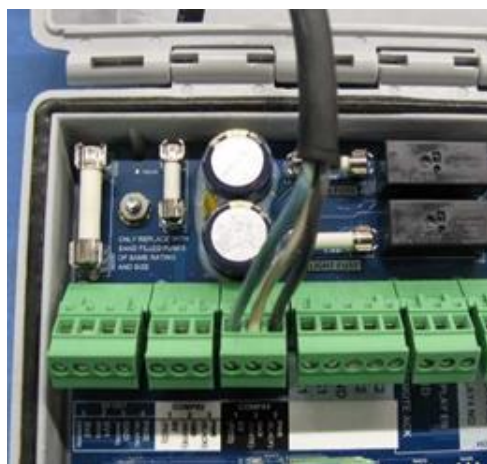
Figure 2-5-4B, Connection Power, Ground, SV
