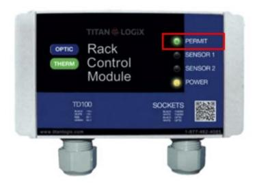
The RCM automatically resets the **permit** light to **green** when the **HH** and **Spill** alarms have been cleared and **inactive** for over **1 minute** while the compartment is **empty**.
