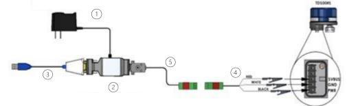
When the transmitter is installed on a truck and programming it through the FINCH II (first two transmitters only)
